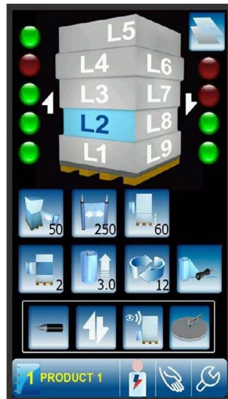
**Strategic Film Placement** allows you to place the film exactly where it has the most impact on load stability and containment. This innovative technology allows you to place bands of film or roped film in critical areas of your loads. Thousands of hours of testing in our labs have shown that putting film in the correct position, with the correct containment force is key to successfully shipping any product.
