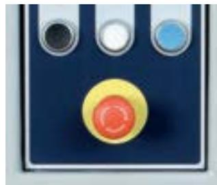
**Emergency stop:** Large button located prominently on control panel stops all machine operations immediately.
