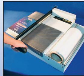
With the film covered product now resting on the work table, close the sealing jaw to form a bag around the product. Product is now in a bag with one open end, and the edge of the film is sealed for the next package.
