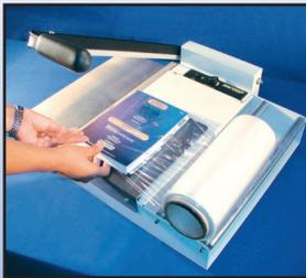
Place the corner of the product on the combination film separator/loading table. Slide the product into the open end of the center-fold film, and into the sealing position. The leading edge of the film was left sealed when the previous package was made.
